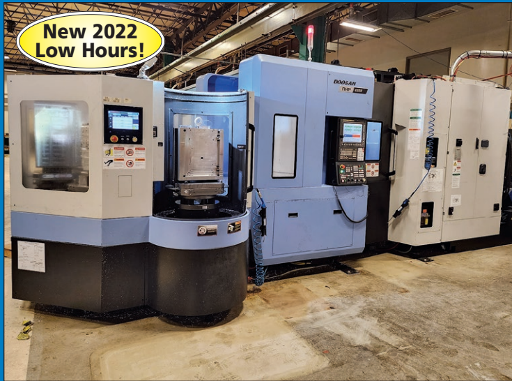
Doosan NHP 4000 CNC Horizontal Machining Center Equipped with 4-Station Doosan RPS 4000 Rotary Pallet System
